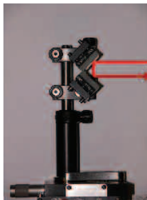
Figure 4.4 The beam exiting the delay line should travel parallel to the incoming beam
