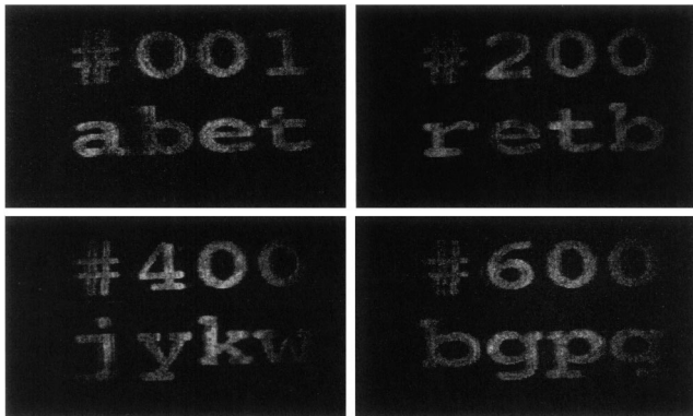
Fig. 4. Samples of reconstructed images from fixed-revealed holograms. The numbers in the pictures are the hologram numbers.
