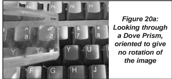
Figure 20: The Dove Prism - Not Rotating an Image
