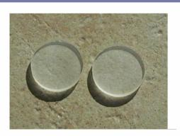
LiF is used for windows, mirrors, and refracting components in the ultraviolet, visible, and infrared. LiF has the lowest refractive index of all common infrared materials. It also transmits ultraviolet radiation more effeciently than any other material, with a transmission range of  $150-6000\,\mathrm{nm}$ .
