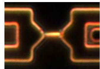
Fig. 4: Single silicon nanowire trapped between electrodes
