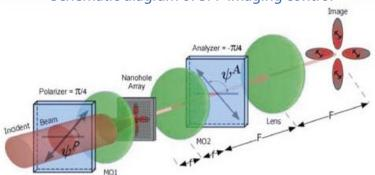
A sample is illuminated using a focused laser. The resulting SPP mode is then imaged onto an InGaAs CCD array via a 4F imaging system.
