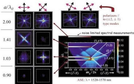
Measurements for cubic arrays of holes in aluminum film on glass substrate. The stitching frequencies appear as horizontal black lines. The SPP images were obtained using four samples .Images of the higher order SPP modes obtained with laser illumination of nanohole arrays.
